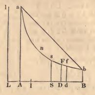
Take S I=S s, and describe a hyperbola passing through a, s, b, to which L l, L B are asymptotes; then as in the former case, the area A a n b B = A L.S B.  $\int \frac{L B}{L A} = L S.S s \int \frac{L B}{L A} = S I.L S \int \frac{L B}{L A}$
